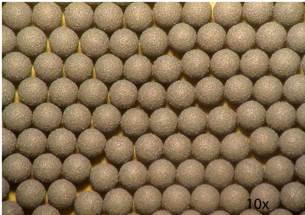
Figure 5: Light optical image of SnHg50 spheres with a Hg content of 1.5 mg.
